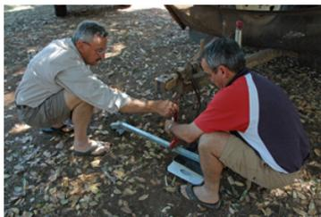
However, some people won't invest in a ball-weight scale, so a set of bathroom scales can suffice, in conjunction with a sturdy piece of wood or steel tube between the scale and the ball receiver. It's necessary to use a load-spreading pad of wood on top of the scale, so you don't damage its upper surface.
