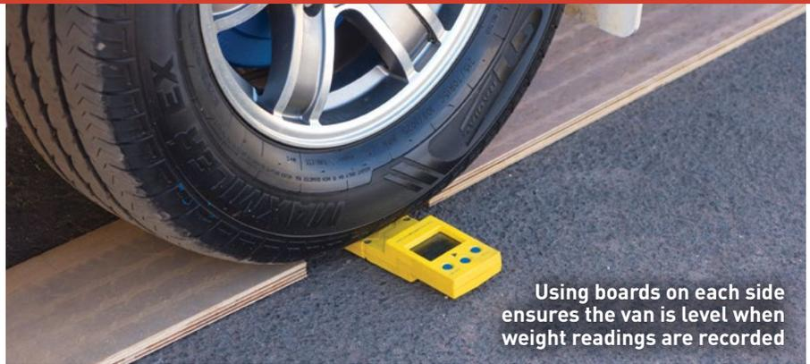
Using boards on each side ensures the van is level when weight readings are recorded
